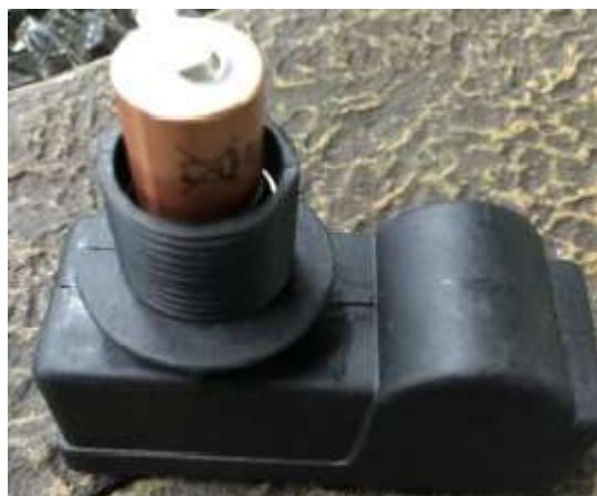
The Cosiconcrete features a piezo ignition that runs on one AA battery . It may happen that after repeated use , the battery runs out . The battery can be replaced as follows :
