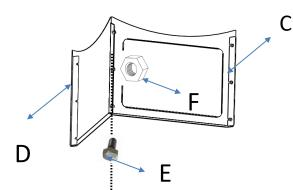
Connect the left panel(D) and rear panel(C) with 3pcs Connect the right panel(D) and rear panel(C) with 3pcs screws(E) and 3pcs nuts (F)
