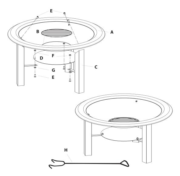
Attach the legs  $(3x \, \mathbf{C})$  with the bolts  $(6x \, \mathbf{E})$ , rings  $(3x \, \mathbf{G})$  and nuts  $(3x \, \mathbf{F})$  onto the bowl  $(\mathbf{A})$  and middleplate  $(\mathbf{D})$ . Place the grill  $(\mathbf{B})$  into the bowl.
