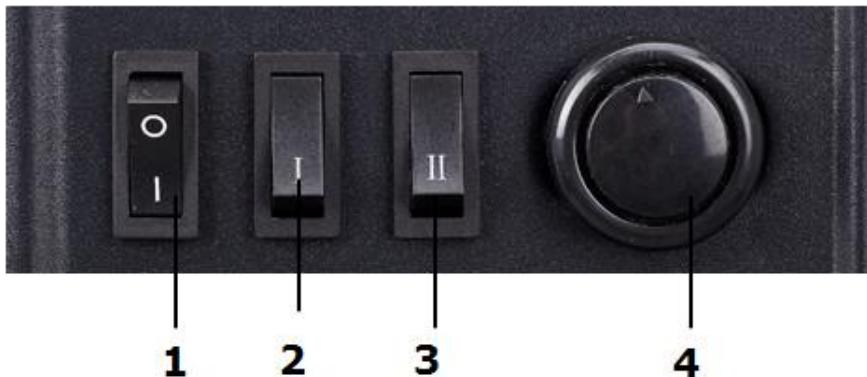
Switch 1: switch on the power supply to the heater and the flame effect (without heating) (**O** depressed is OFF - **I** depressed is ON).
